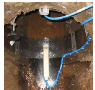
Air-ultrasonic, water-ultrasonic and hydrostatic measurement – for detection of the entire discharge range e.g. to investigate channel efficiency
